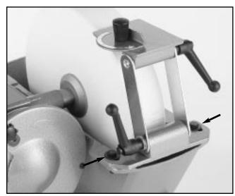
Figure 3. Bolts to mount tool rest.
